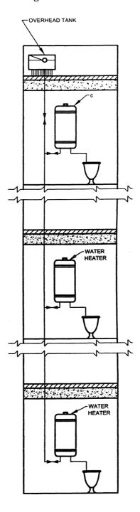
Figure 12 Non – Pressure Type Installation
