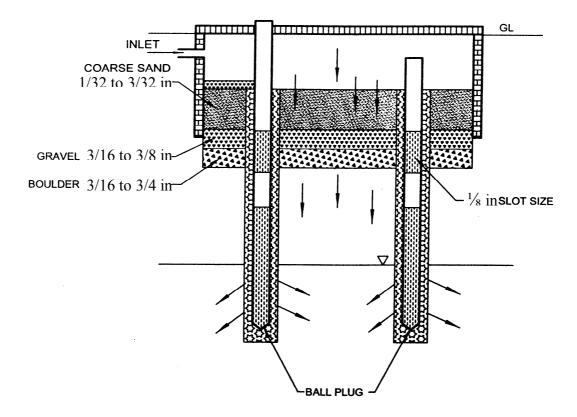
Fig. 5d.18 Artificial Ground Water Recharge Structure
