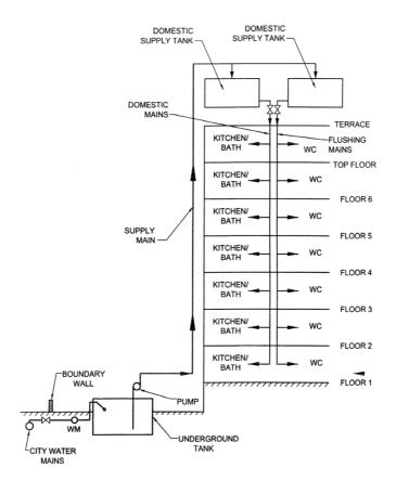
Figure 8 Overhead Tank Distribution
