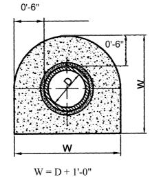
where D is external diameter of the pipe
