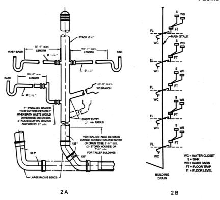
Figure 2 Single Stack System – Main Feature Of Design
