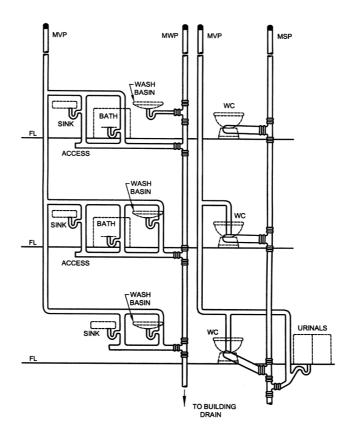
Figure 4 Diagram Of Two-Pipe System
