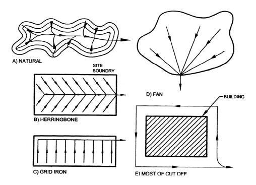
Fig. 19 Details Of Drainage System
