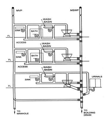
Figure 3 Diagram Of One-Pipe System
