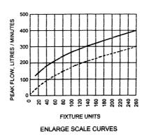
FIG. 5D.13 PEAK FLOW LOAD CURVES
