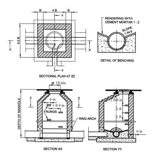
Fig. 5d.14 Detail Of Manhole (Depth Less Than 3 Feet)
