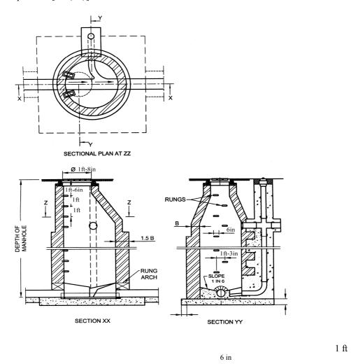
**NOTE** – Wall thickness have been indicated in brick length to provide for use of modular bricks or traditional bricks. In the Fig. B = one brick length, 1.5B = one and a half brick length etc.
