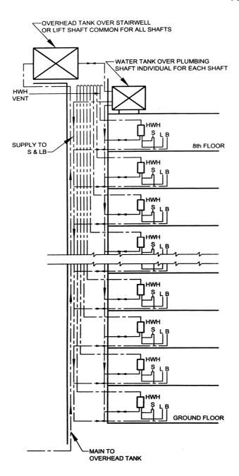
Figure 9 Installation For 8 – Storeyed Building
