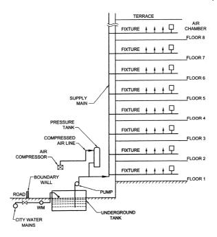
Figure 7 Hydro-Pneumatic System
