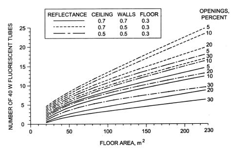
Figure 2: Supplementary Artificial Lighting for 40W Fluorescent Tubes
