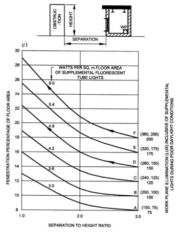
Figure 3: Nomograph for Daylighting and Suplemental Lighting Design of Building
