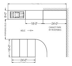
Figure 2.11.5 Parking Stalls which Cannot Park by Reversing
