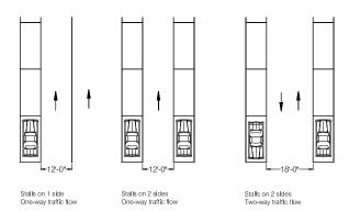
Figure 2.11.6 Dimensions of Parallel Parking Aisles 30°-60° Angled Parking Aisle
