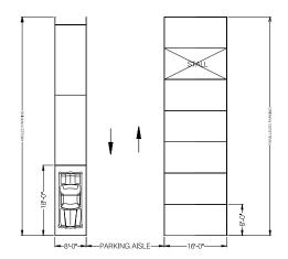
Figure 2.11.3 Position of Parking Stalls and Required Dimensions (Above figure)
