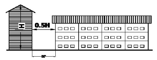
Figure 2.11.2 Schematic Figure Showing Spacing of Row Blocks,
