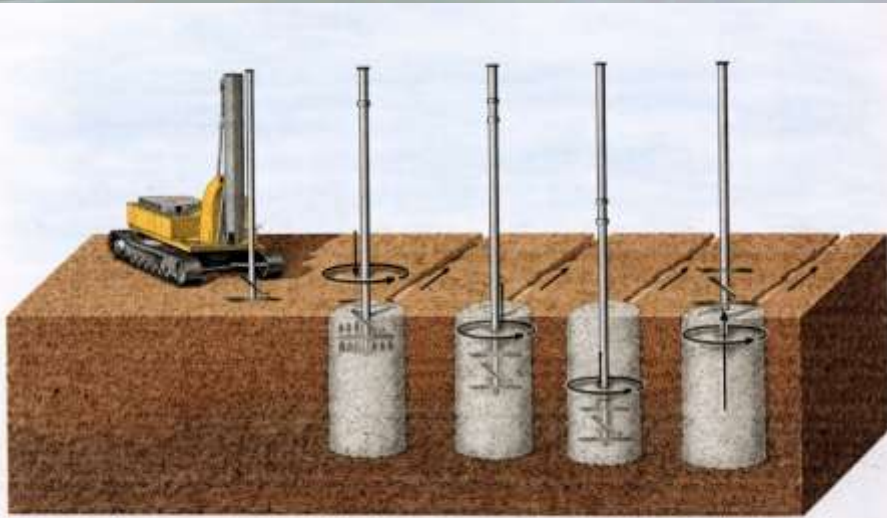
Figure 119. The deep soil mixing process (Hayward Baker, Inc.).
