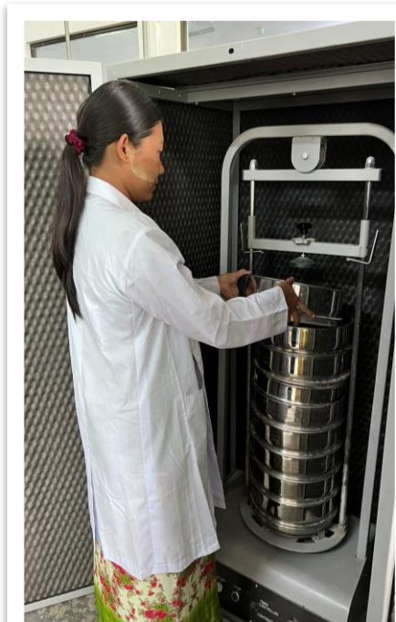
Sieve Analysis with Sieve Shaker
