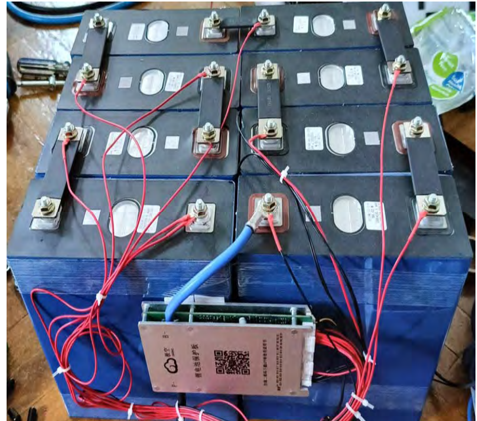
LiFePo4 battery with Jikong BMS control unit
