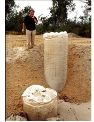
Confining capability of high strength geotextile encasement
