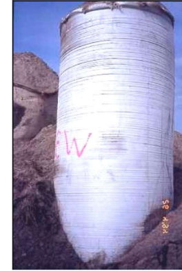
Confining capability of high strength geotextile encasement
