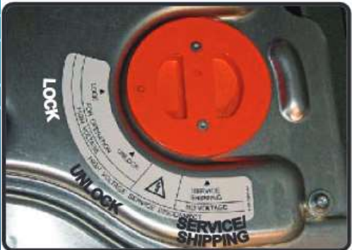
High-Voltage Service Disconnect Switch Shown in LOCK position.
