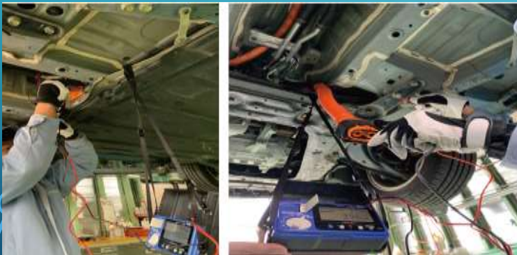
(LHS), Insulation Test for HV Battery Side
