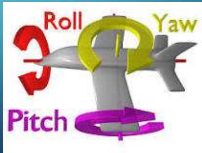
The Rudder Controls Yaw
